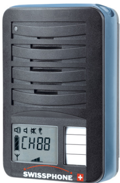
Paging device manufactured by Swissphone used for emergency communications with fire departments.
